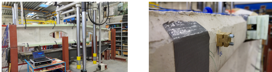
Figure 1. The experimental setup of the modal test. (a) Side view of the experimental setup. (b) One of the connections for the FBG sensors.
