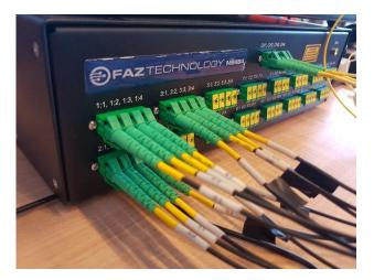
Fig. 4: FAZ 64 channel interrogator, using an optical multiplexer system.
