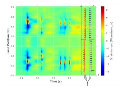
Fig. 5: Road monitoring example: Horizontal strain (color map) as a function of sensor position (vertical axis) and time for a truck passing a FO strainline buried into a tarmac layer.
