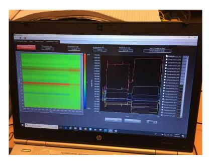
Fig.9: Display of the FO Strain measurement system during Factory Acceptance Test. The left panel displays a complete pile as strain color map, the right panel gives conventional strain versus time display for a group of sensors.
