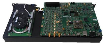
FAZ 14 Interrogator, optics (left) and electronics (right) boards
