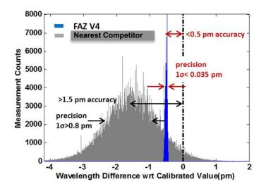
Fig. 3: FAZ I4, precision and accuracy compared to the nearest competitor (**Compared System**). A single FBG under controlled conditions is measured for a long time, the individual measurements are sampled into a distribution. The deviation from the "true" measurement is defined as precision, the width of the distribution (the scatter) is defined accuracy.
