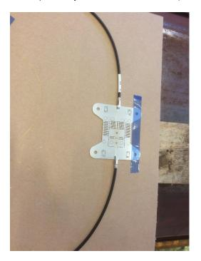
Fig. 6: Fugro Strain sensor, basic sensing element without cover and protection. The combination of optical fiber and spring "multiplier" is clearly visible, the fiber runs between the two black cable ends across the spring structure and is mounted using mineral glass solder. The round "spots" are the markers for the actual welding points to the to be monitored structure.
