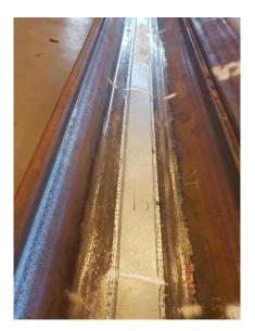
Fig. 8: Covered and waterproofed strain sensor line ready for field deployment.
